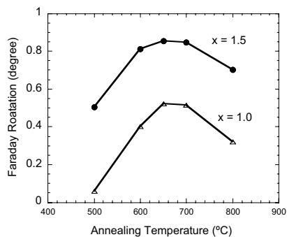
**Fig. 3** Annealing temperature dependences of Faraday rotation of  $\text{Y}_{3-x}\text{Bi}_x\text{Fe}_5\text{O}_{12}$  films measured with  $\lambda = 500 \text{ nm}$ .
