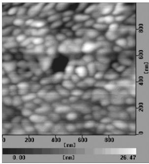
**Fig. 4** AFM image of  $\text{Y}_2\text{BiFe}_5\text{O}_{12}$  films with thickness of 400 nm.
