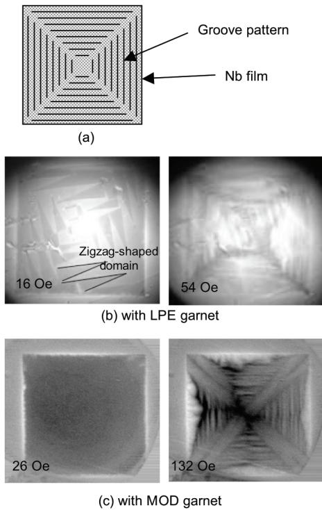
**Fig. 5** (a) A schematic drawing and (b),(c) MO images of Nb film with groove patterns. A size of the Nb film is  $0.9 \text{ mm} \times 0.9 \text{ mm}$ , and a pitch of groove with a width of 4  $\mu\text{m}$  is 4  $\mu\text{m}$ . (b) and (c) were measured by using the LPE-grown and the MOD-grown garnet, respectively.
