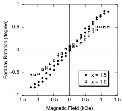
**Fig. 2** Magnetic field dependences of Faraday rotation of  $\text{Y}_{3-x}\text{Bi}_x\text{Fe}_5\text{O}_{12}$  films measured with  $\lambda = 500 \text{ nm}$ .
