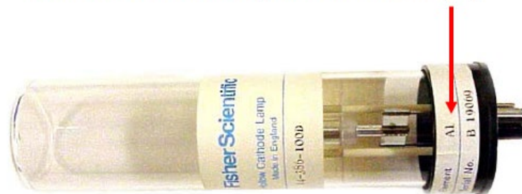
A hollow cathode lamp for Aluminum (Al)
